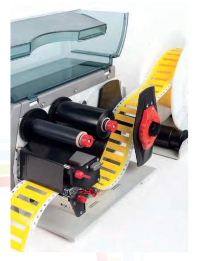
Supplied in a "ladder format", sleeves are held horizontally between two hole-punched polyester strips and offers ease of printing and kitting.
